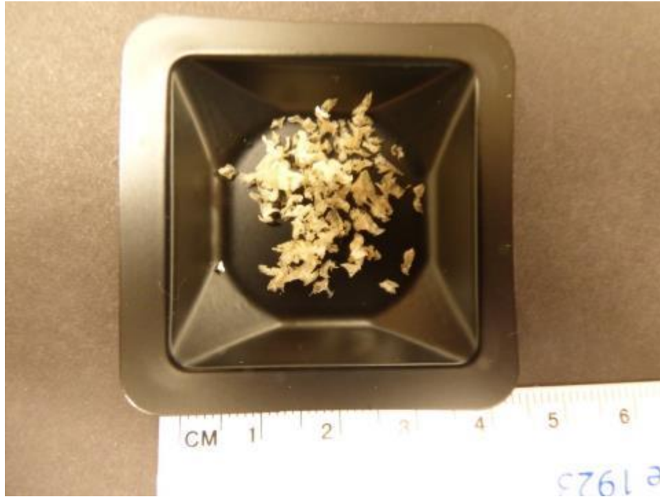
Figure 4 Decellularized ECM has been lyophilized at -104.3^{\circ}\text{C} and 14mTorr for approximately 48 hours
