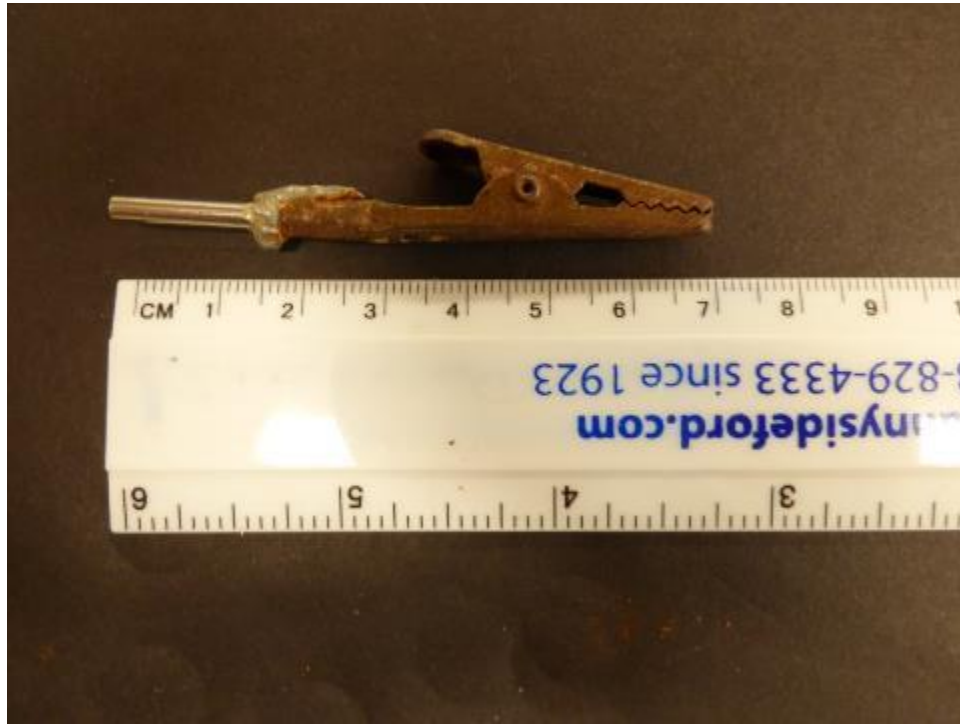
Figure 7 Modified Steel Alligator Clips for Microthread Tensile Testing.
